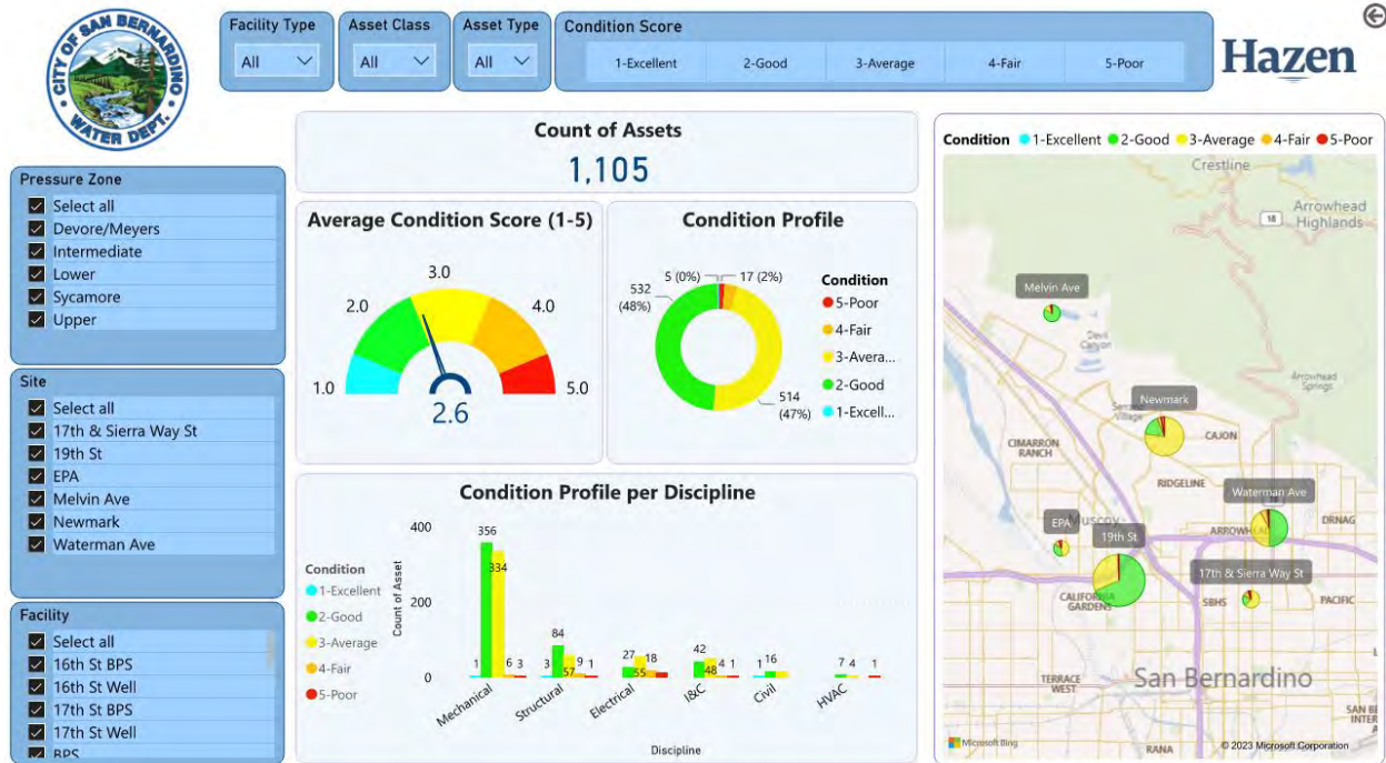
Figure 11-5: A Snapshot of Condition Assessment Results in the Asset Management Dashboard
