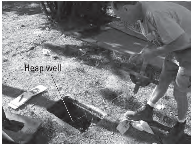
Figure 29. Heap well (1S/4W-3Q1) in the San Bernardino area, California. Heap well, being measured by USGS Hydrologic Technician Kimball Stumpf and located on the edge of the former marshland, is used to estimate ground water rising into Warm Creek (fig. 21) and underflow from the Bunker Hill basin (fig. 28).
